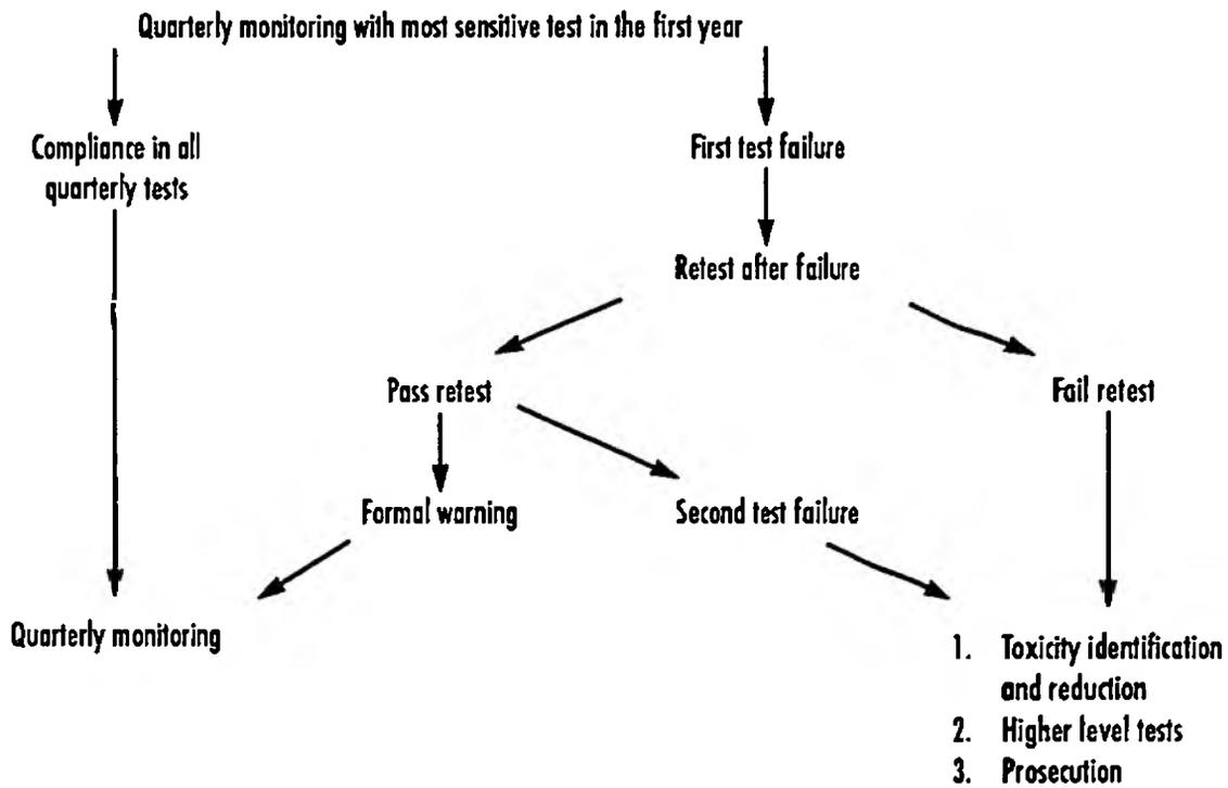
**Figure 2.5 Compliance monitoring of effluents with 'calibrated' screening test consent limits or limits derived using the most sensitive tests**
