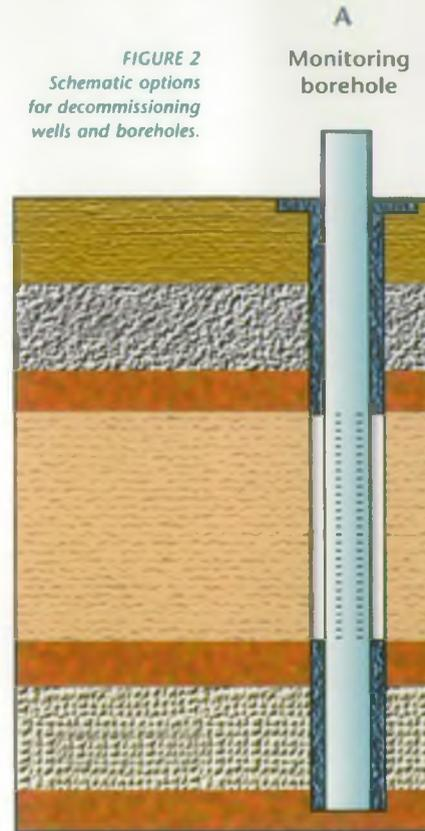
in Section 4 (above) indicates that the boreholes intersect important aquifer units (in terms of resource and quality), and are constructed so that representative groundwater samples may be collected or water levels measured. The ideal borehole construction and completion is dictated by the geological strata encountered and its intended use. Boreholes which intersect a single aquifer unit may be cased through the unsaturated zone, but open hole
