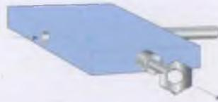
Pull out to release the lock barrel, this will release the spring loaded sliding lockbolt and allow the handle to turn
