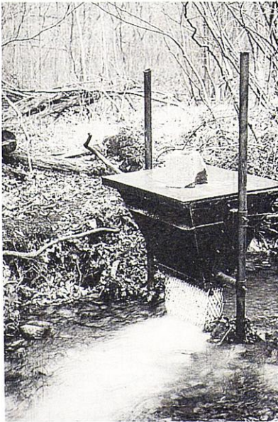
A basket-doser in the Mosquito Creek watershed, Pennsylvania, U.S.A. Limestone powder can be seen as it is washed out of the doser loaded with limestone briquettes.
