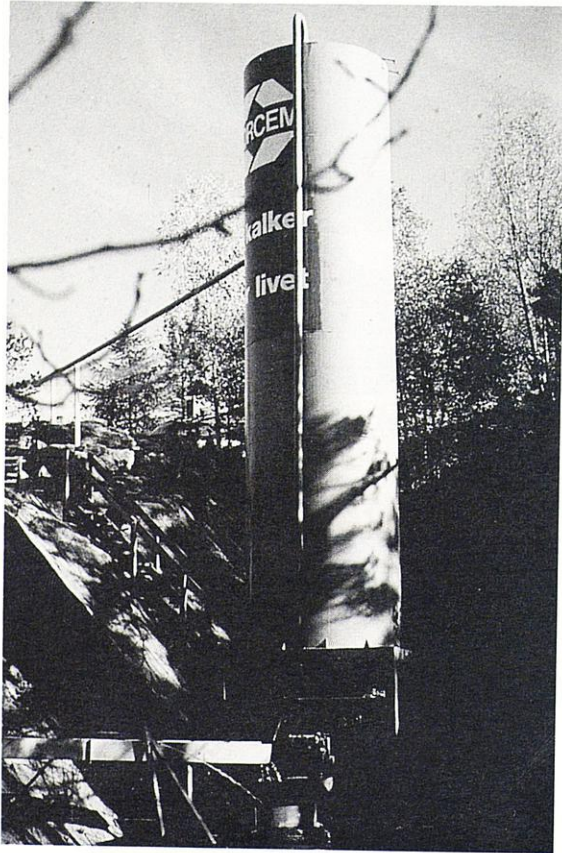
A typical stream-dosing machine which dispenses finely-powdered limestone from the cylindrical hopper via a water-powered mechanical device.
