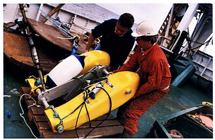
Revolutionary new gear: the open 'cod end' with the video camera housing on the right side, and Dr Jens Christian Holst with the catamaran and transmitter.
