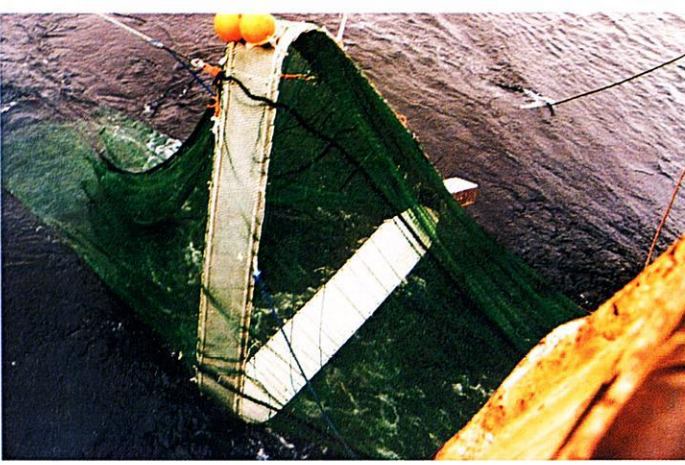
Revolutionary new gear: the open 'cod end' with the video camera housing on the right side, and Dr Jens Christian Holst with the catamaran and transmitter.
