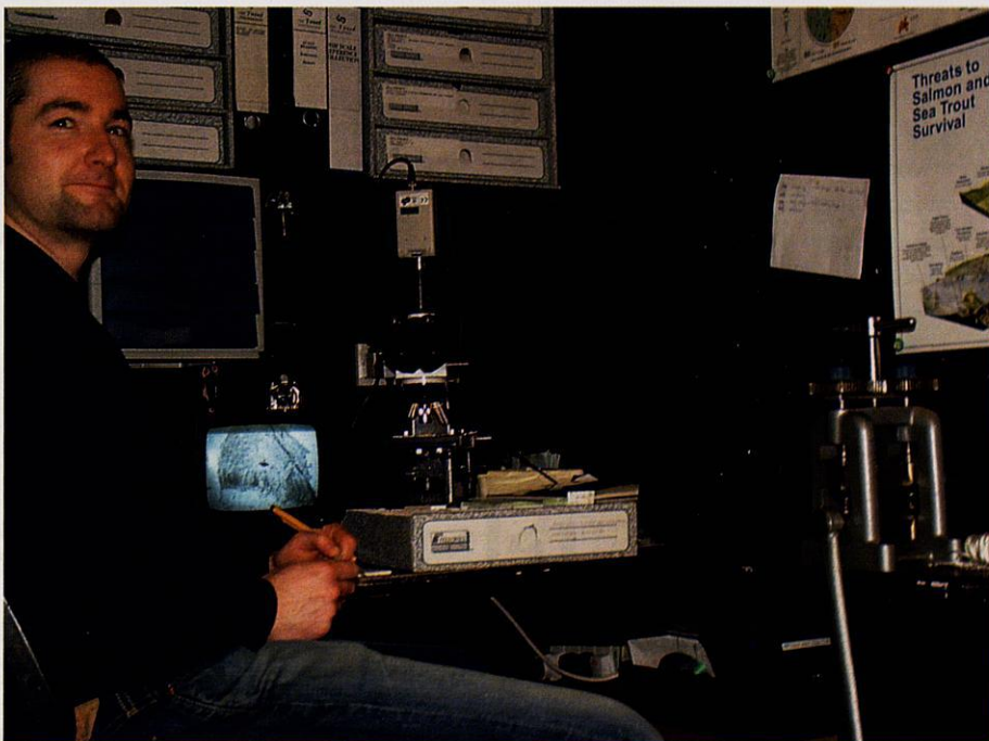
Barry Wright, the Tweed's scale-reader. On the right is the press used to make impressions of scales onto clear plastic for reading – such impressions are cleaner than the original scales. The digital microscope is in the centre with a scale on its screen beside it.
