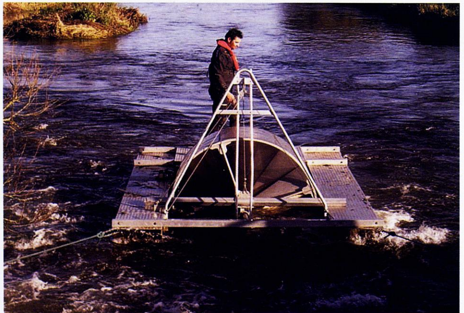
Rotary Screw Trap being operated on the River Frome
